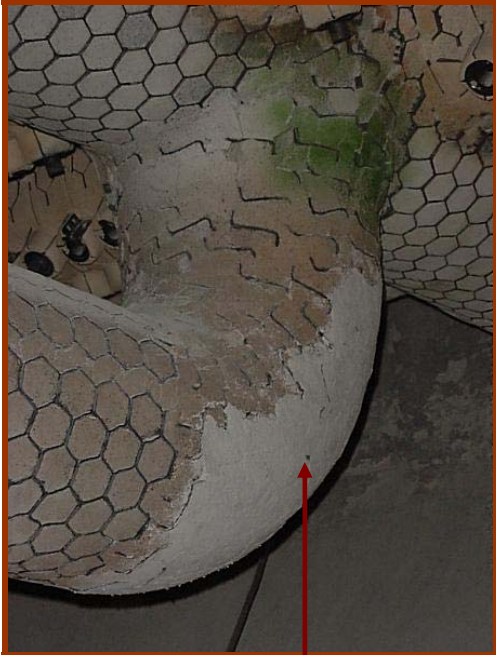
Fig. 08 ACTCHEM 75 + 3% s/s fibre on Air Grid Elbow
